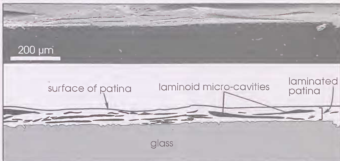
Figure 8. SEM image and annotated line diagram of a cross-sectional view of patina on glass (sample A3) showing laminated patina, and laminoid micro-cavities.
